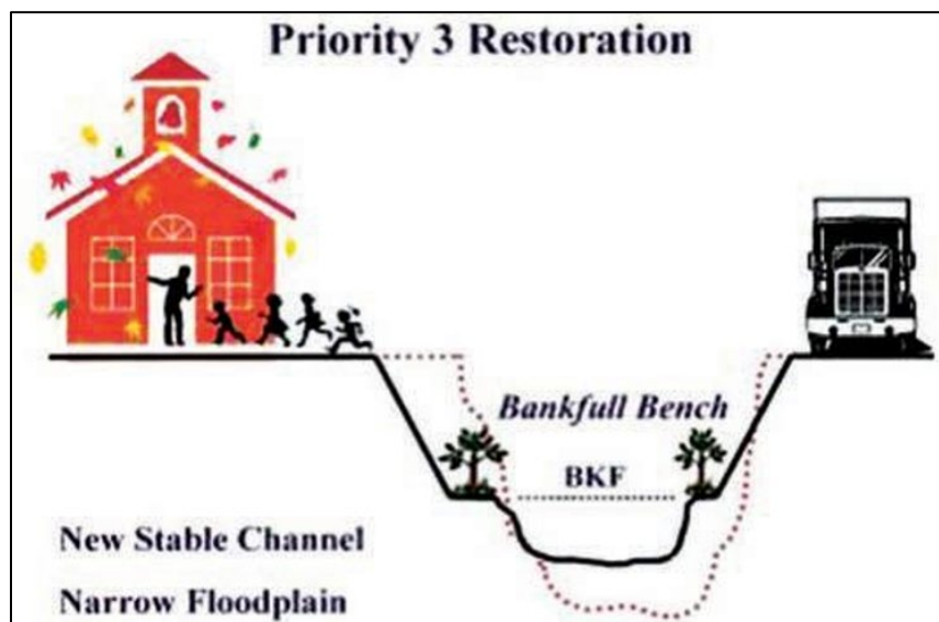
Figure 6.28 Conceptual cross section of Priority 3 restoration (Doll et al. 2003)
