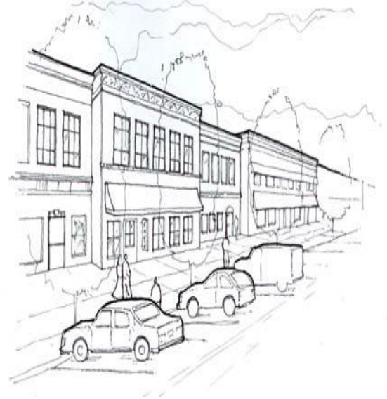
Figure 7-2. Long building facades should use variations in building mass while still presenting a consistent streetscape.
