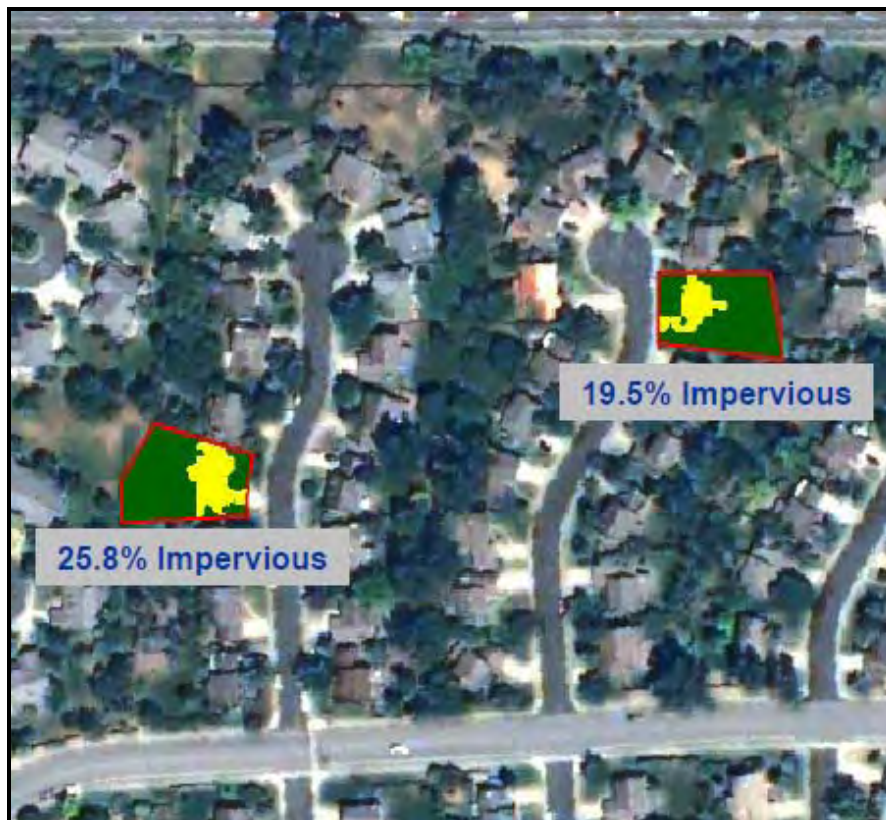
Figure 2-33. Measured Percent Impervious Cover for Individual Residential Lots
