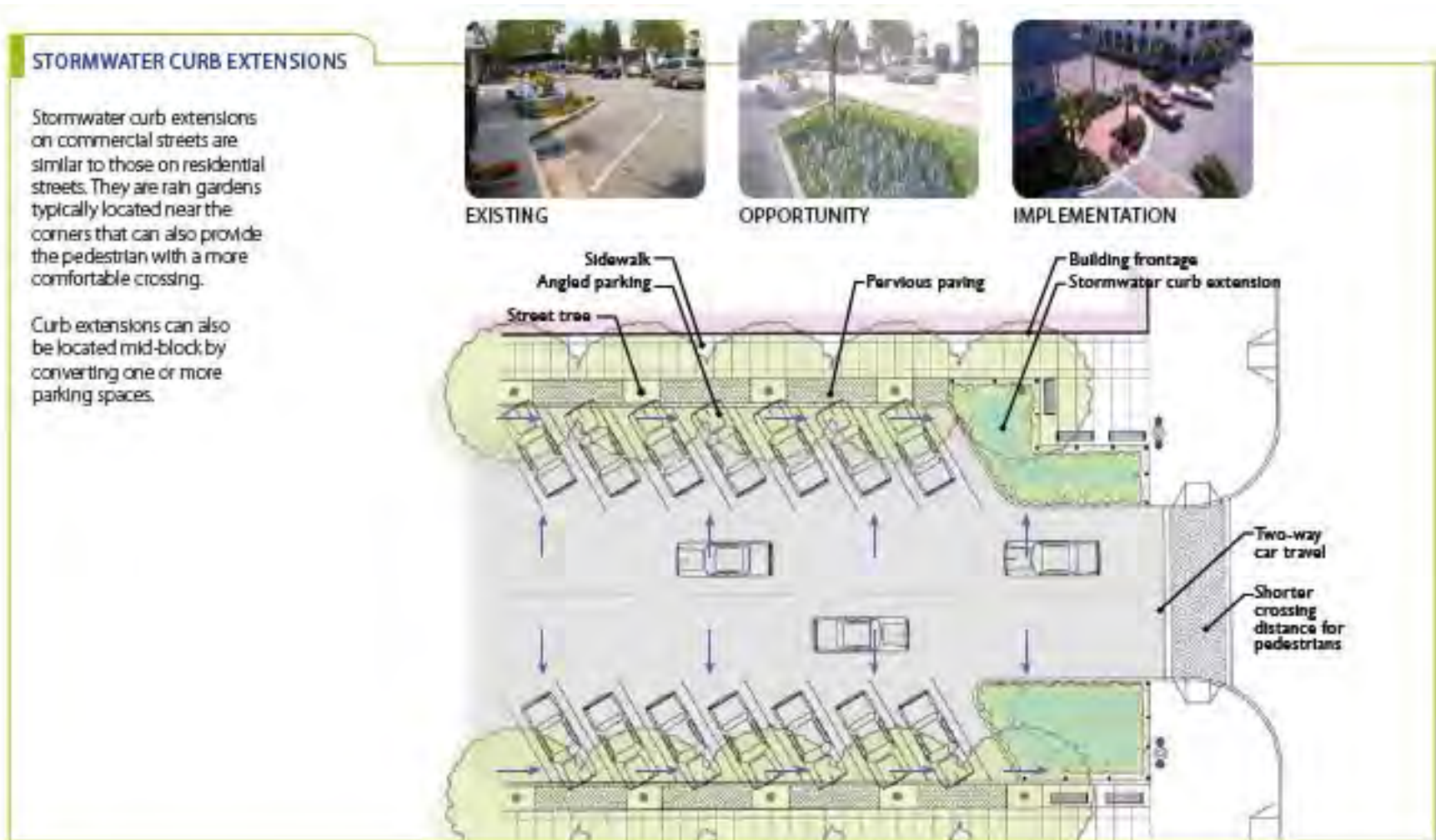
Figure 6-30. Example Application of Stormwater Curb Extensions in a Commercial Parking Lot (Source: EPA's 2008 Managing Wet Weather with Green Infrastructure)
