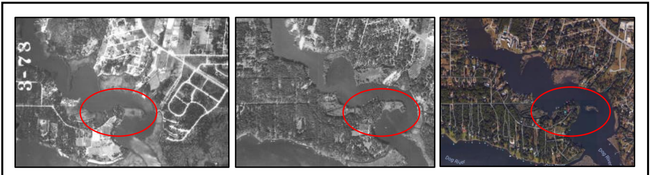
Figure 5.2.11: Aerial imagery representing the narrowing or reduction of spits (point bars) located on Dog River near the Neshota subdivision for 1952 (left), 1974 (middle), and 2016 (right) (UA, 2016; Google Earth, 2016)
