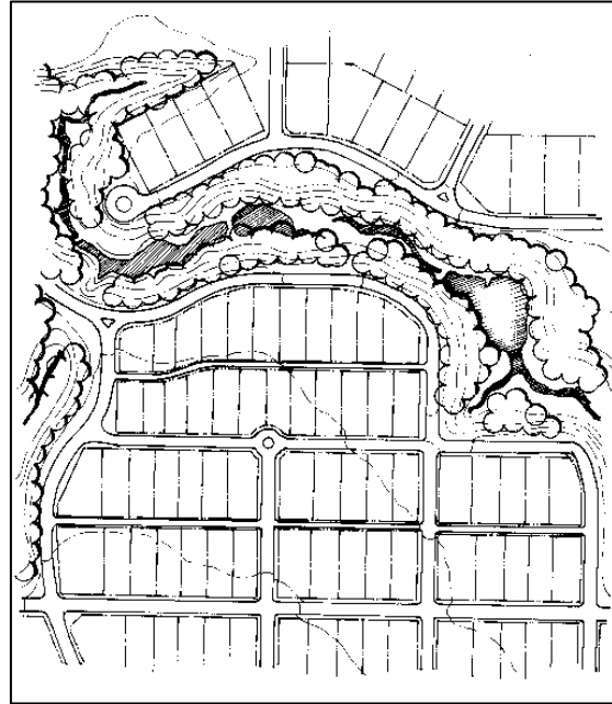
Figure 5.15 – Street layout exception due to natural, topographical, or environmental features causing interruptions in the street network. The exception to the street standard still maintains the street connections and maximum block limits.
