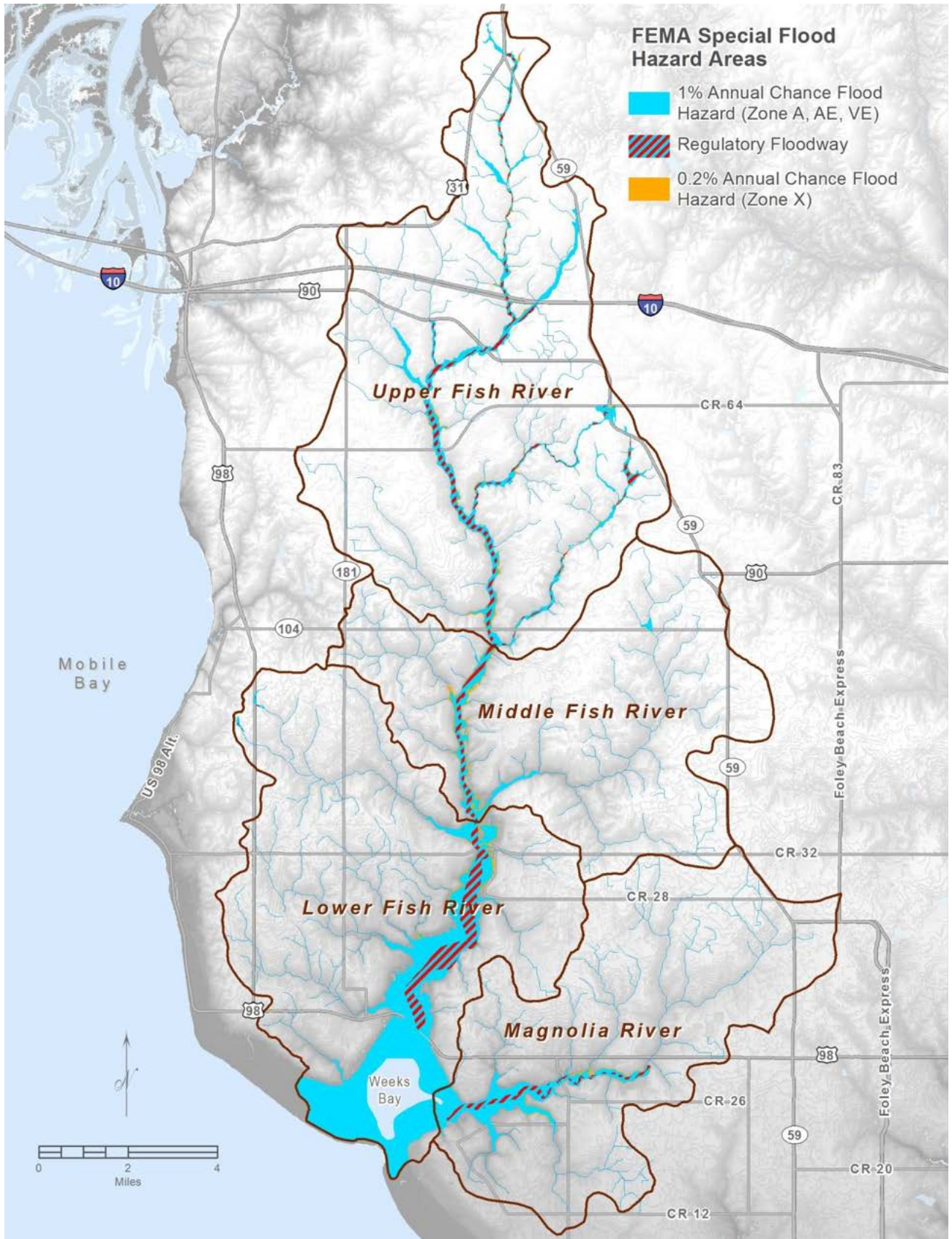
Figure 2.11 Federal Emergency Management Agency Flood Zones within Weeks Bay Watershed
