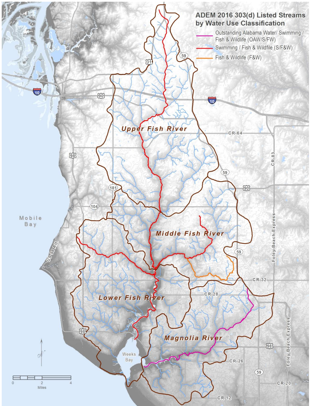
Figure 3.1 ADEM Stream Classifications and 303(d) Stream Segments Note: All smaller blue-colored streams are classified as Fish & Wildlife (F&W)
