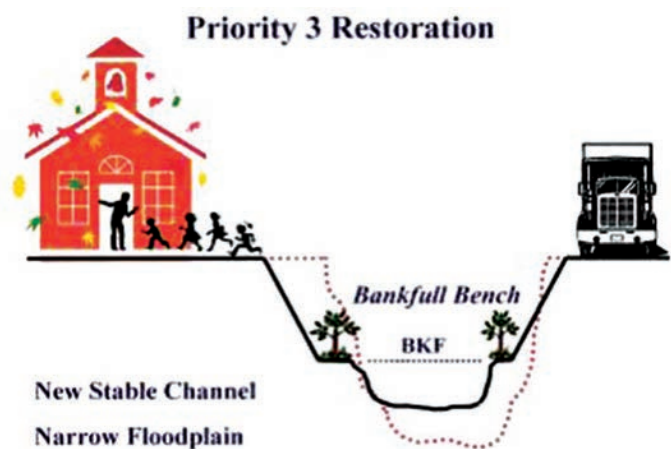
Figure 6.15: Conceptual cross section of Priority 3 restoration (Doll et al. 2003)
