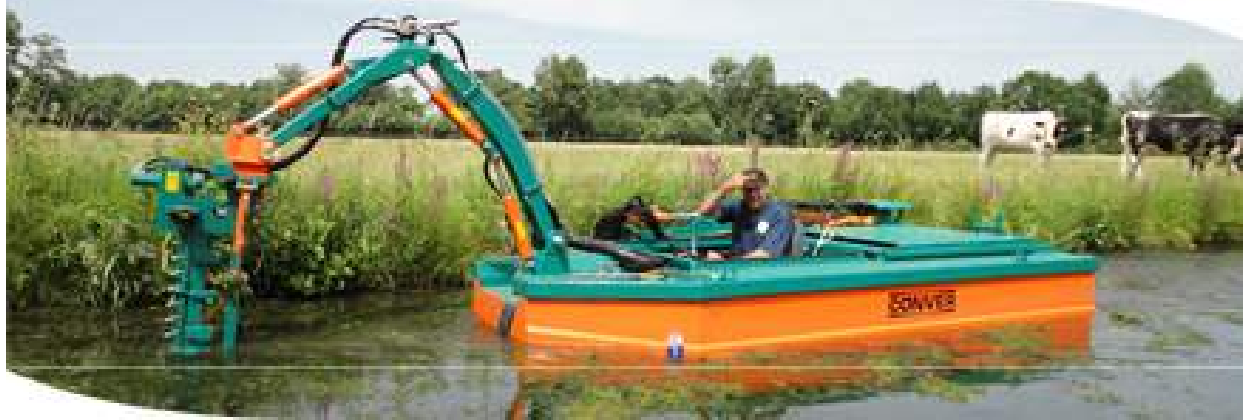
Figure 6-5 The Conver boat is well suited for shallow water vegetation removal and dredging ( http://flaqim.com/harvester_boats.html )
