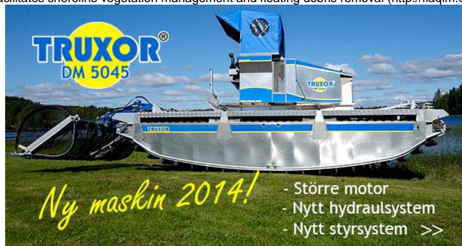
Figure 6-4 Truxor Amphibian Toolcarrier facilitates shoreline vegetation management and floating debris removal ( http://flaqlm.com/harvester_boats.html )
