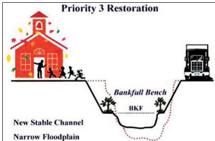
Figure 6.29 Conceptual cross section of Priority 3 restoration (Doll et al. 2003)
